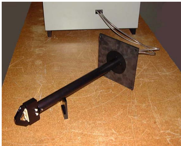
Figure 3 Imacc fiber-optic linked probe for monitoring in industrial ducts/stacks.
