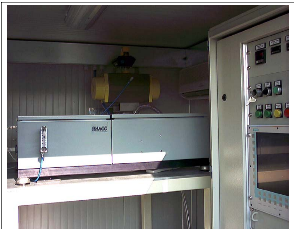
Figure 1 Imacc Cross-stack FTIR on an industrial incinerator in Europe.
